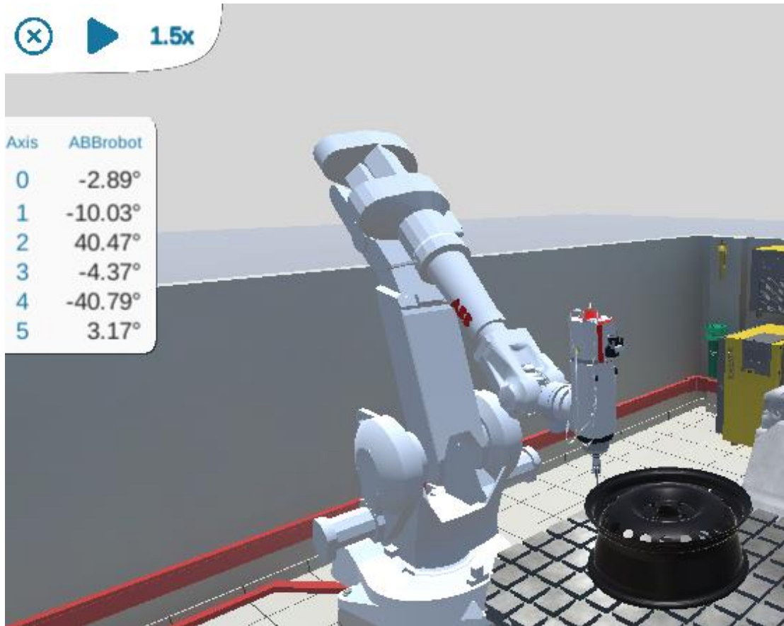
Figure 20 - New functionality of the VR application after academic teachers' intervention (speed range simulation button and angles of the ABB robot arms for all of the axis)
