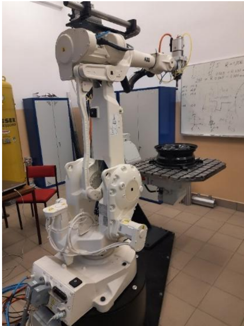
Figure 12 - View of ABB robot with workpiece - steel wheel rim of a vehicle
